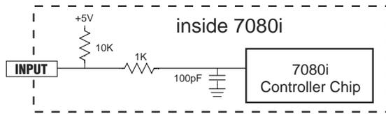
Schematic Diagram of Inputs 1 - 4, cw jog and ccw jog)
