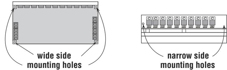
The amplifiers in the 7080i generate heat. To operate the drive continuously at maximum power you may need additional heat sinking or forced air cooling. Never use your drive in a space where there is no air flow or where other devices cause the surrounding air to be more than 50 C. Never put the drive where it can get wet or where metal particles can get on it.
