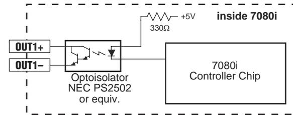
**Schematic Diagram of 7080i Output Circuit**
